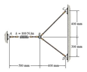
The Force in The Spring: The spring stretches  $s = l - l_0 = 0.5 - 0.2$ = 0.3 m. Applying Eq. 3 - 2, we have
