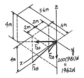
**3–56.** The ends of the three cables are attached to a ring at A and to the edge of a uniform 150-kg plate. Determine the tension in each of the cables for equilibrium.
