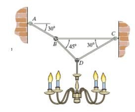
Equations of Equilibrium: First, we will apply the equations of equilibrium along the x and y axes to the free-body diagram of joint D shown in Fig. (a).
